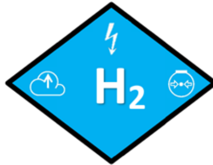
Figure 5. A symbol developed by CTIF for FC vehicle powered by compressed gaseous hydrogen [38]
