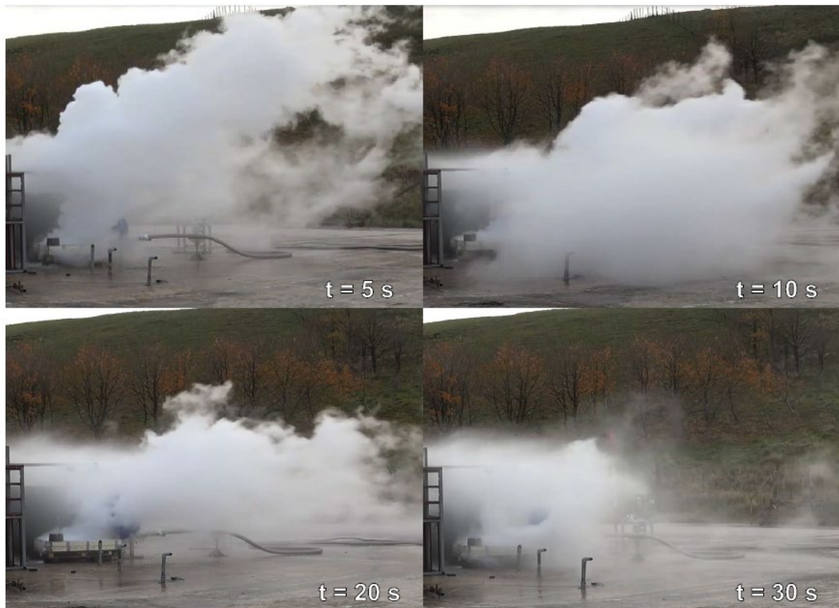
Figure 10. Vapor production after 5, 10, 20 and 30 s of water spray impingement.
