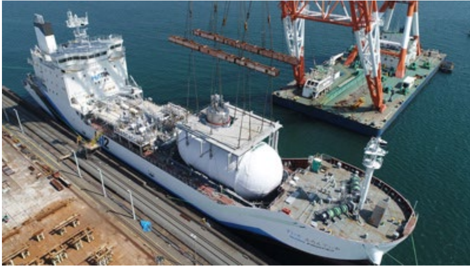
Figure 35. SUISEO FRONTIER, the world's first LH 2 carrier ship launched in 2019 with LH 2 storage tank [75].
