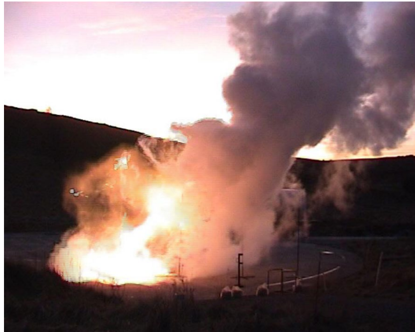
Figure 14. Ignition of the LH 2 vapor cloud during low wind conditions (no secondary explosion).
