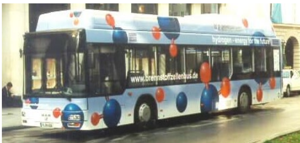
Figure 44. MAN hydrogen-driven fuel cell bus of 1996 with LH_2 storage tanks
