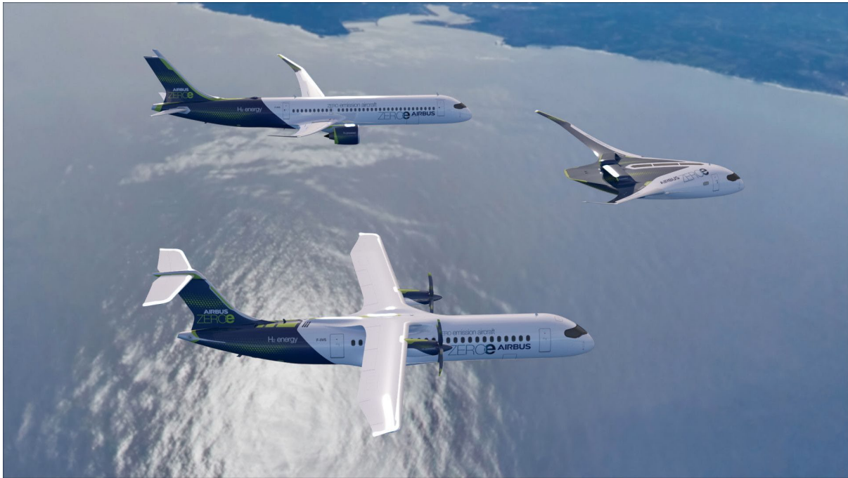
Figure 53 Airbus ZEROe concept aircrafts. Turbofan, 'blended-wing body' and turboprop designs from up down.
