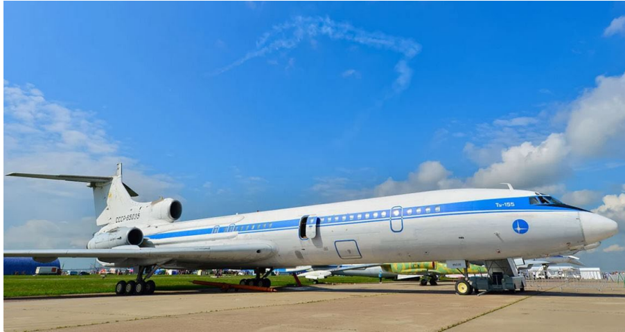
Figure 51. Tupolev 155 “Flying Laboratory” of 1988 with the central engine fuelled by LH 2 or LNG [91].
