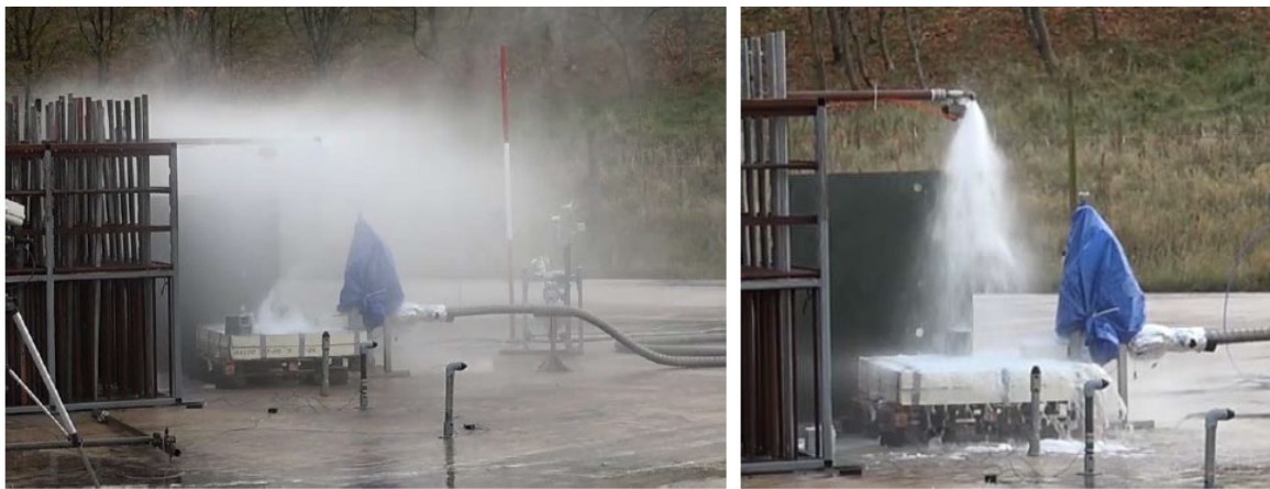
Figure 9. Experimental facility for rapid phase transition investigation. Left: fully developed water spray from sprinklers. Right: water jet application into the centre of the tray (right).
