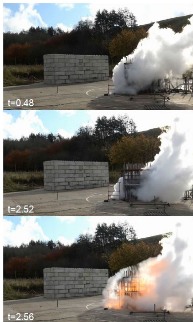
Figure 21. Pictures showing sudden gust immediately prior to ignition for test with release: p = 1 bar, d = 12 mm, and wind velocity = 2m/s.
