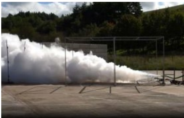
Figure 7. LH 2 large-scale release and delayed ignition (5 bar - 12 mm; PRESLHY project - HSE).
