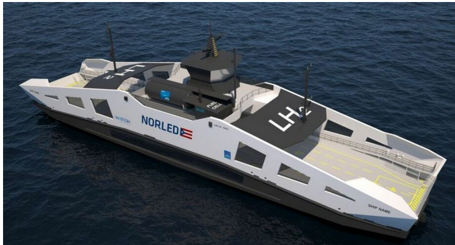
Figure 48. On-deck arrangement of LH 2 storage, fuel cell and vent mast on the NORLED ferry [85].
