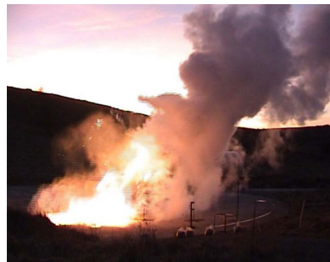
Figure 7. LH 2 large-scale release and delayed ignition (5 bar - 12 mm; PRESLHY project - HSE).
