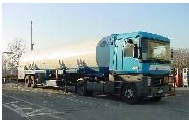
Figure 15. A road tanker operated by Air Liquide for conveying LH 2 to the end-user.
