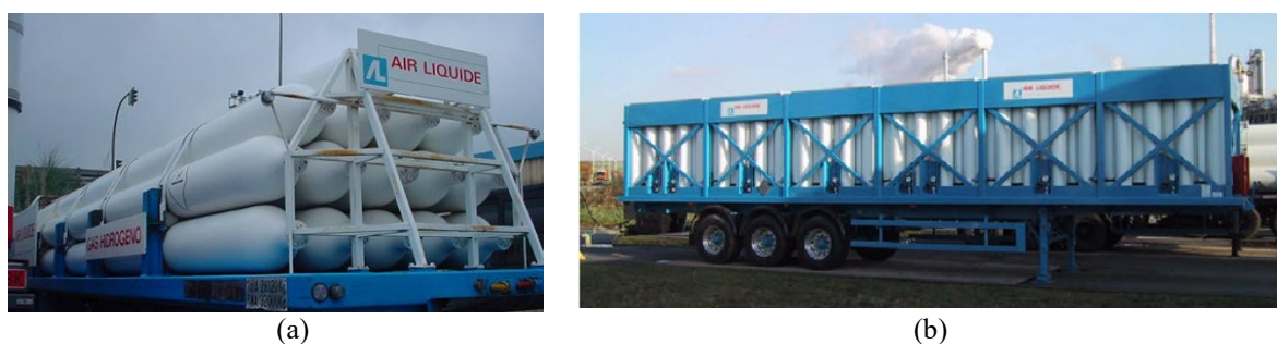
Figure 13. Two types of CGH 2 trailers operated by AirLiquide in Europe: (a) tube trailer carrying 2,000 to 3,000 Nm 3 of hydrogen and (b) composite cylinder trailers carrying 6,200 Nm 3 of hydrogen.
