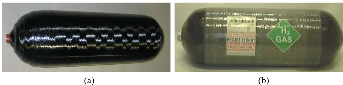
Figure 6. 700 bar cylinder prototypes developed and tested within the STORHY European project: (a) Type III technology, (b) Type IV technology.
