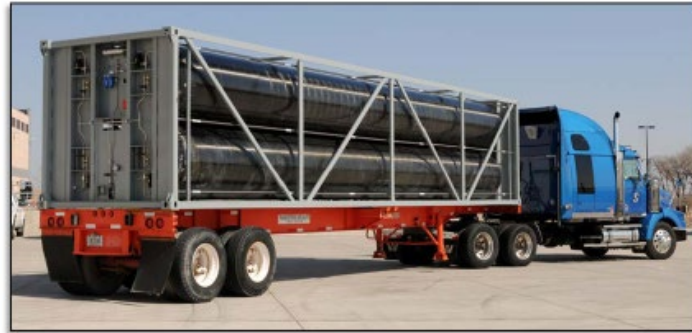
Figure 14. A trailer carrying four composite tanks developed by Lincoln Composites.
