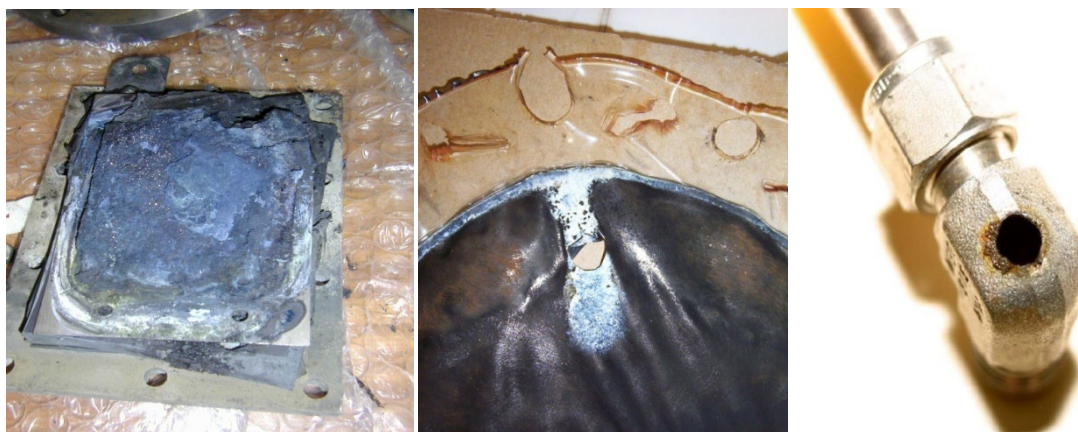
Figure 23. Damaged parts of high pressure PEM electrolyser.
