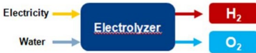
Figure 32. Principle of electrolysis process.
