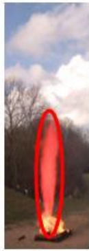
Equivalent Ø: 3,1 mm H2 length flame: 5,5 m
