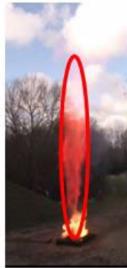
Equivalent Ø: 3,1 mm CNG length flame: 8 m
