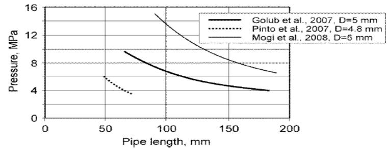
Experimental data on pressure limit of spontaneous ignition of hydrogen release into air in pipes of different length.
