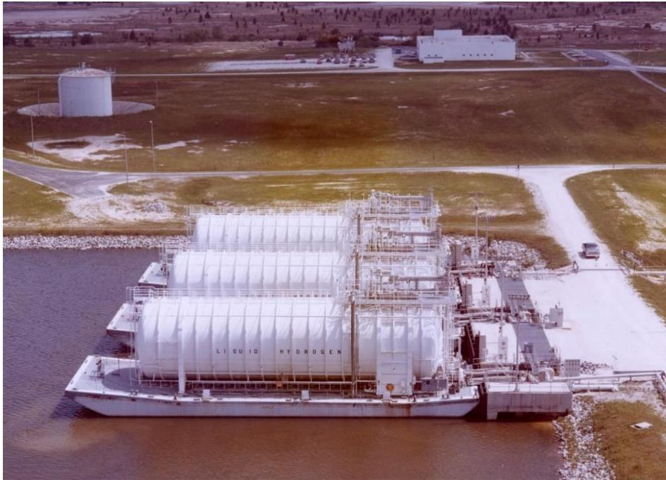
NASA liquid hydrogen barge fleet
