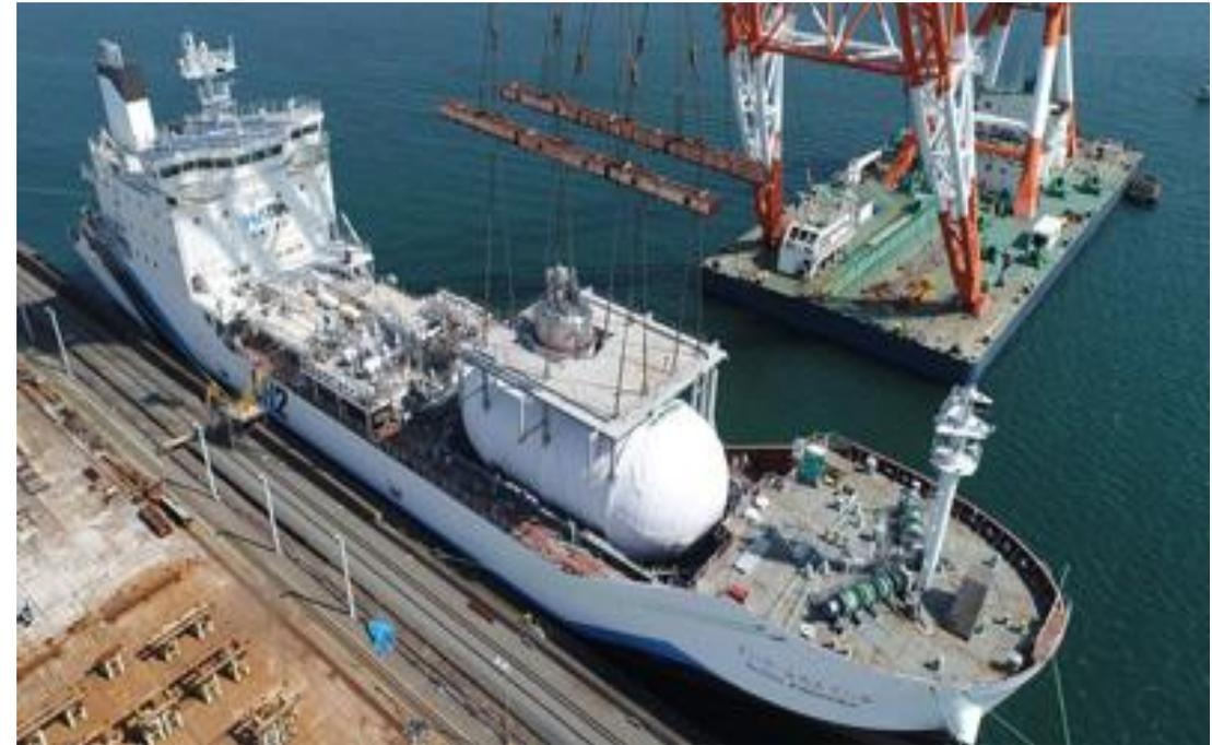
The world's first LH<sub>2</sub> carrier ship SUISEI FRONTIER
