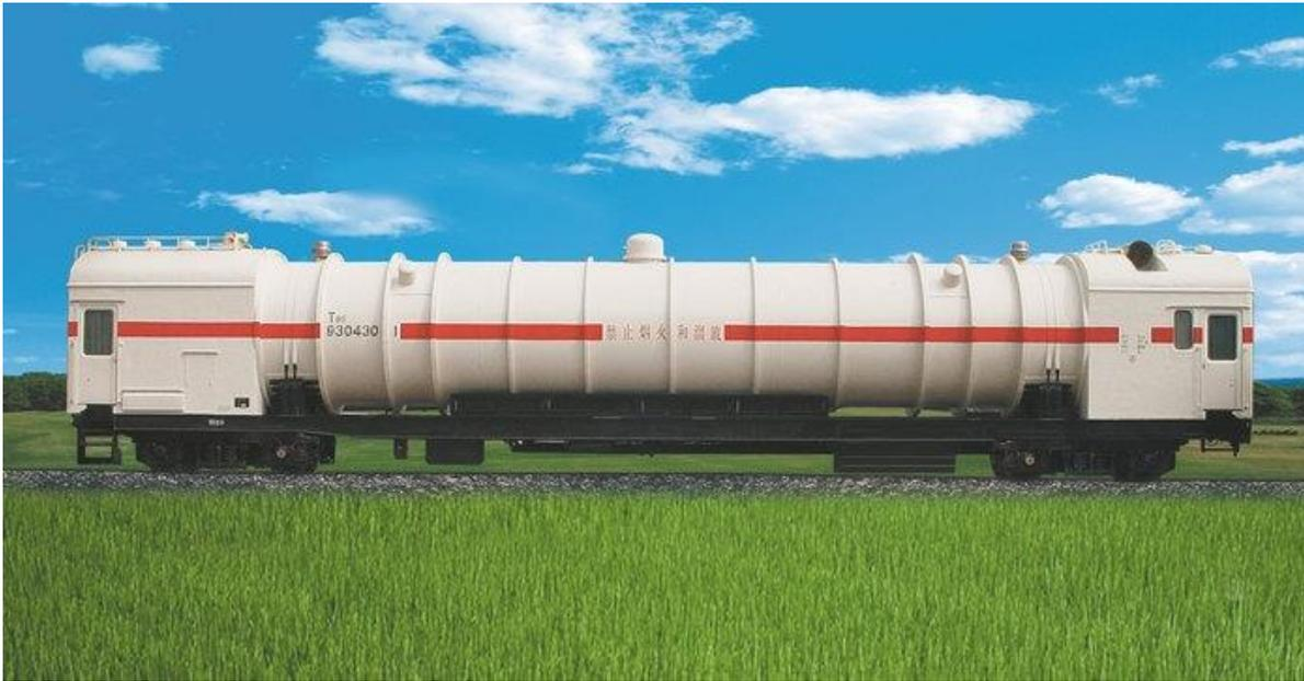
The design of a rail car for liquid hydrogen (and other cryogenic commodities) transports manufactured by the Chinese company CRRC Xi'an Co.,Ltd., a traditional enterprise in railway transportation equipment. The thermally insulated tank with a total volume of 85 m<sup>3</sup> to carry a payload of 5 t can be used for direct loading, unloading, or transfer filling.
