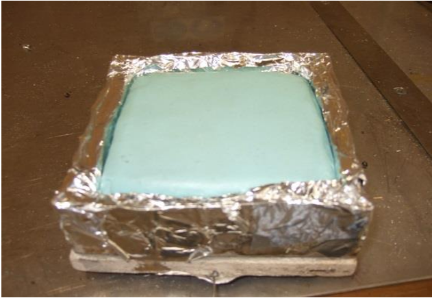
Intumescent coating before the fire exposure
