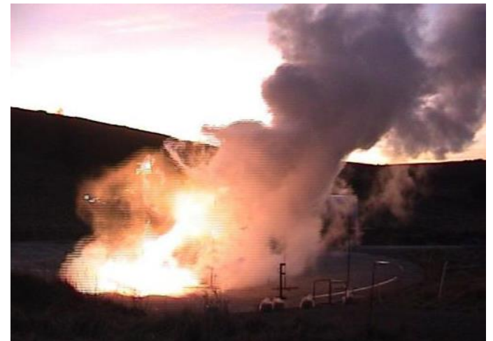
LH 2 vapour cloud ignition, HSL experiment, UK [2]
