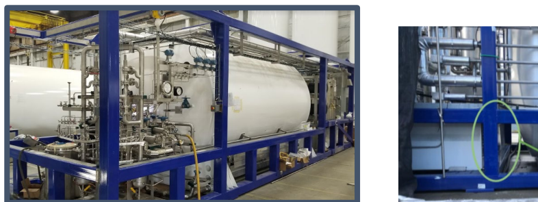
Figure 6. Crash protection (in blue) at the bottom.
