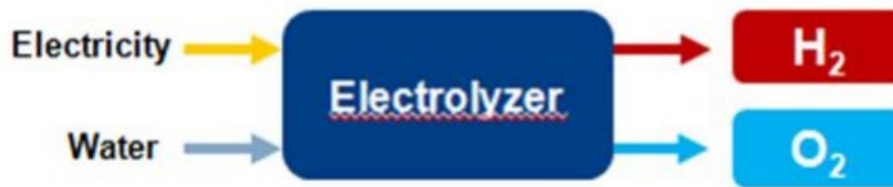
Figure 32. Principle of electrolysis process.
